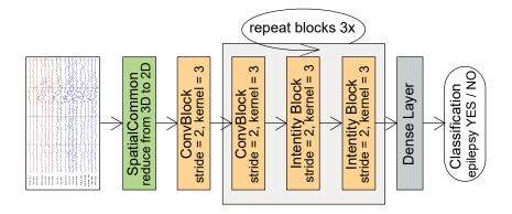
Figure 14: Residual network for end-to-end training (BasicResNet).
