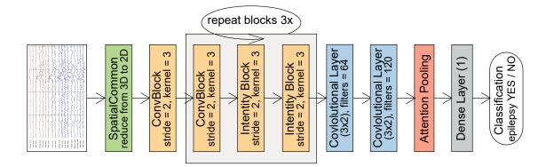
Figure 15: Residual network with Attention Pooling (AttentionResNet).
