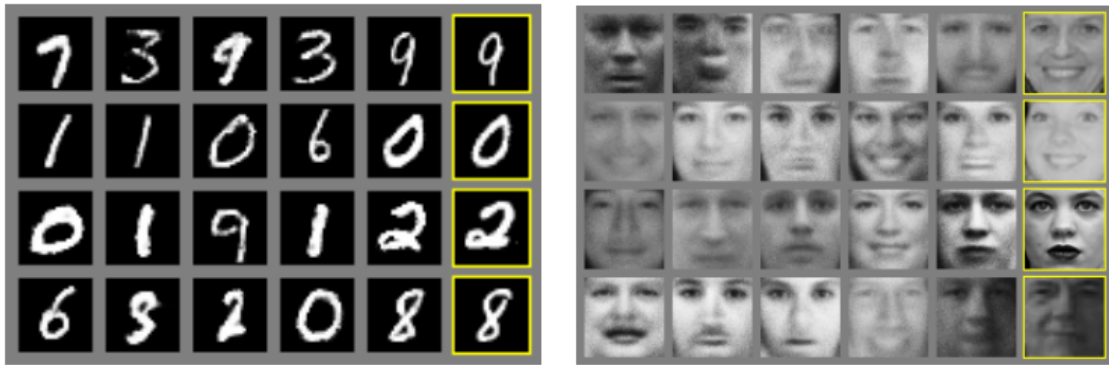
Figure 1.10: Here are some examples of data created by Generative Adversarial Networks. The networks were trained using two datasets, MNIST and Toronto Faces Dataset (TFD). In each set of examples, the rightmost column shows real data closest to the generated data in the neighboring columns. This demonstrates that the network creates new data rather than just copying what it has already seen. [5]
