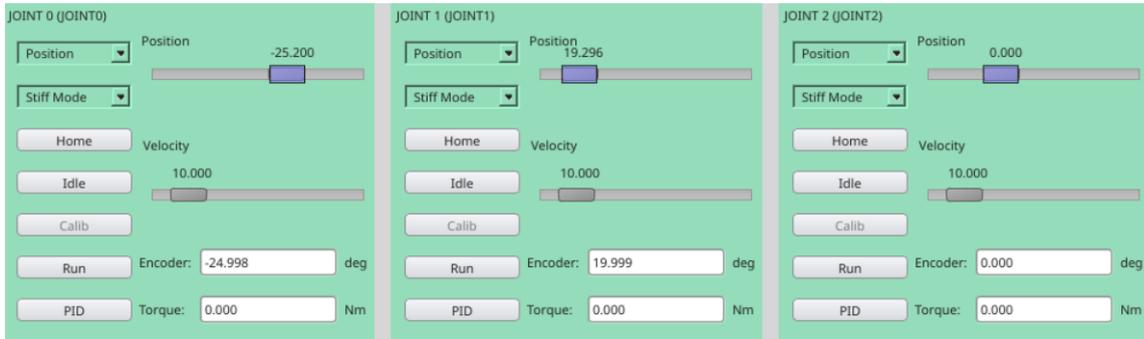
**Fig. 2.3** An example of how the user interface of `MotorGui` looks. For the sake of clarity, only the first three joints are shown.
