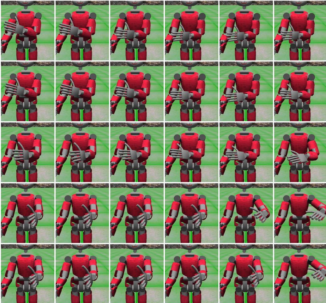
**Fig. 5.1** Visualization a 6 x 5 neurons of SOM representing the left forearm positions the network learned. Topological organisation of the weights can be observed.
