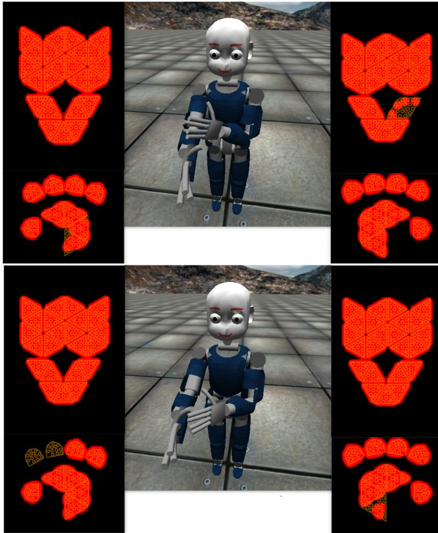
**Fig. 5.9** Comparison of the original proprioceptive configuration (upper image) with predicted configuration (lower image) using touch data.
