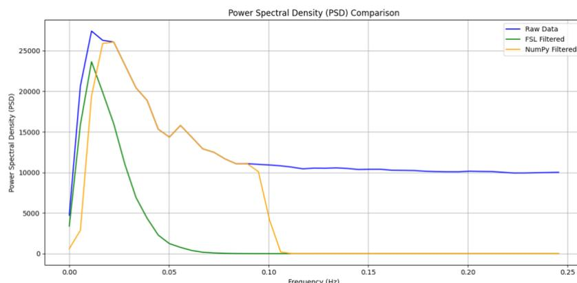
**Figure 2.2.** Comparison of power spectral density (PSD) across different preprocessing approaches. The blue line represents the raw data, the green line shows data filtered using FSL’s default band-pass filtering, and the yellow line represents data filtered using a NumPy implementation.
