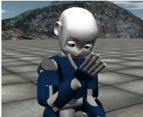
Figure 20: The iCub looking at the palm centre of its right hand. The figure illustrates the data collecting process. For randomly generated values of the robot’s head joints, we collected corresponding angles of the right head joints that move the palm to the position where the iCub is looking at. In Experiment 1 we used two joints controlling the head’s horizontal and vertical movements. In Experiment 2, two joints moving with eyes are used instead.
