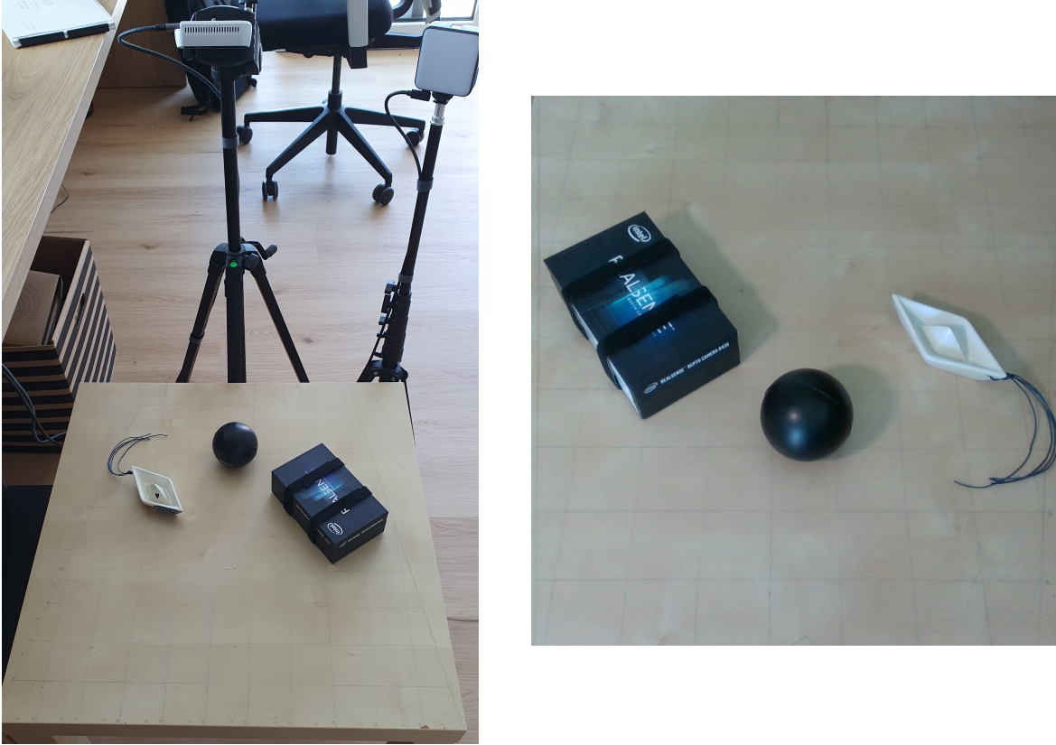
(a) Experimental setup with an RGB-D stereo camera mounted in an oblique overhead configuration, viewing the workspace from above and in front.
